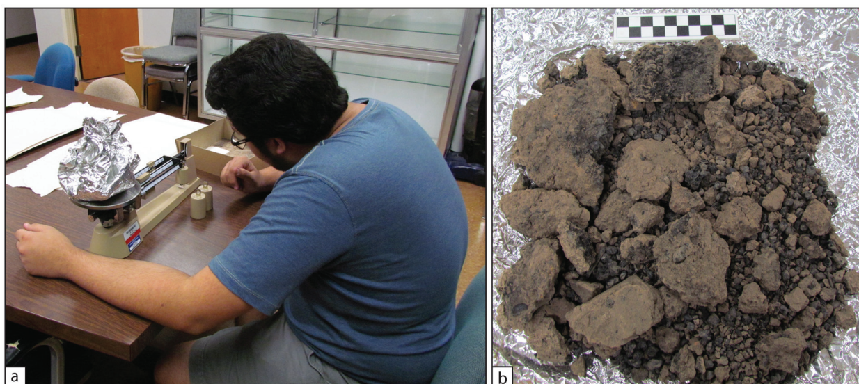
Figure 3. (a) Soil being weighed on a standard triple-beam balance and (b) one section of soil to be floated.
